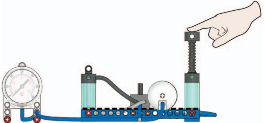
Test how many times can you extend and retract the piston rod when using 1 bar of pressure.
